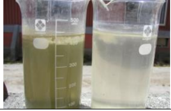
Cow manure, antiseptic solution, milking parlor: Mixed wastewater treatment
